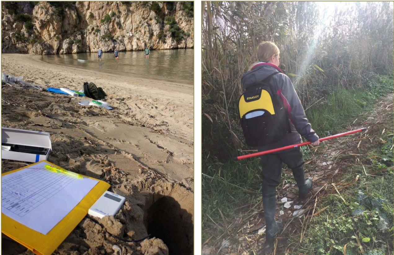
**Figure 4:** Sampling sediments from Voidokilia beach to assess the extent of microplastic pollution (left). Sampling water from Gialova lagoon wetland for nutrient analysis (photos: Michael Valahas).
