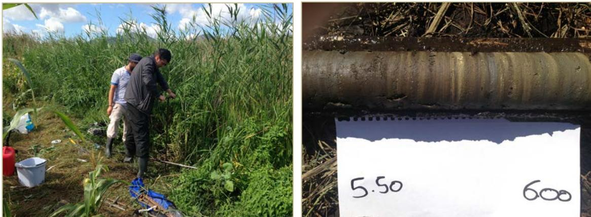
Figure 3: Coring with Russian corer in Ag. Floros.
