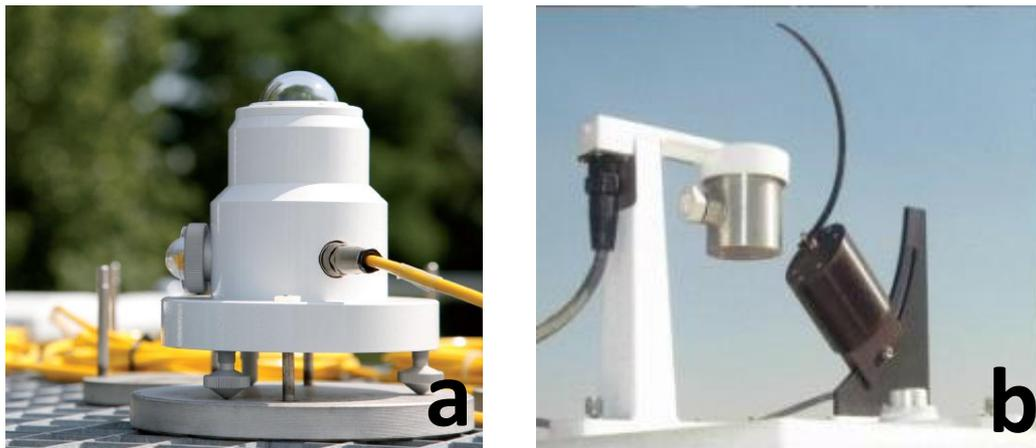
Figure 1: a) UV instrument for measurements of the Erythemal and the UVA irradiance levels, b) MFR Radiometer for measurements of diffuse and total visible solar irradiance and aerosol Optical Depth retrieval
