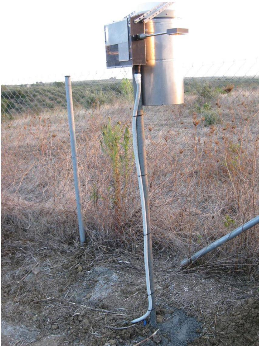
Picture 1: Rain sampler installed at Mouzaki meteorological station
